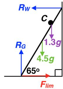
**Working:**  $F_{limG} = \mu R_G$  so we need to find  $F_{limG}$  and  $R_G$ .
