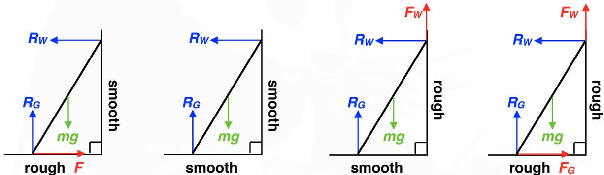
The second and third diagrams could never be in equilibrium because there is no horizontal force to the right to counteract the normal contact force at the top of the ladder.
