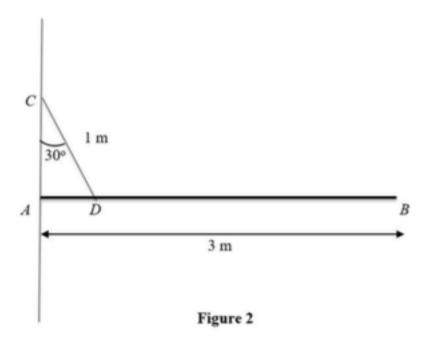
A beam AB, of mass 20 kg and length 3 m, is smoothly hinged to a vertical wall at one end A.
